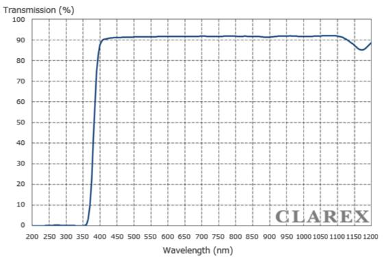
\* These are our experimental measured values in 1.0mm thick.
